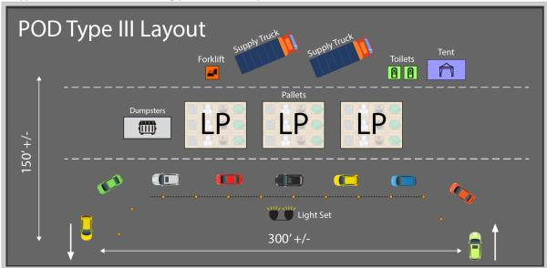
POD Type III layout. It is 300 feet by 150 feet. There are three loading points. Cars are driving in a straight line in between a light set and the loading points. There are dumpsters to the left of the loading points. Behind the loading points is a forklift, two supply trucks, two portable toilets, and a tent.
