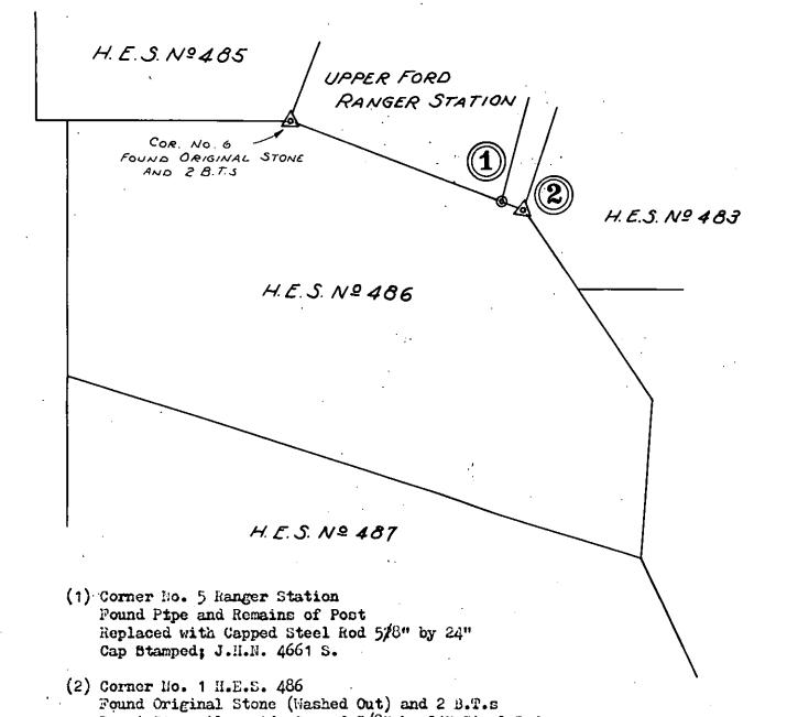
Reset Stone Alongside Capped 5/8" by 24" Steel Rod
