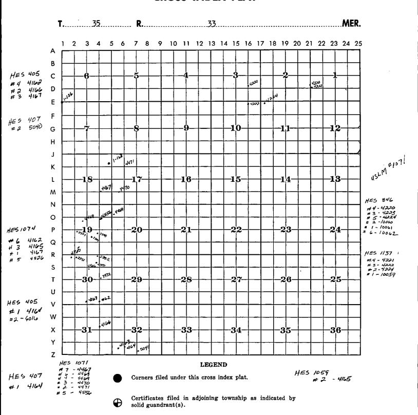
Each corner certificate is identified by an alphabetical-numerical coordinate number which is derived from the system shown on the township diagram. For example, the quarter-corner between Section 5 and 6 is identified as Corner C-5.
