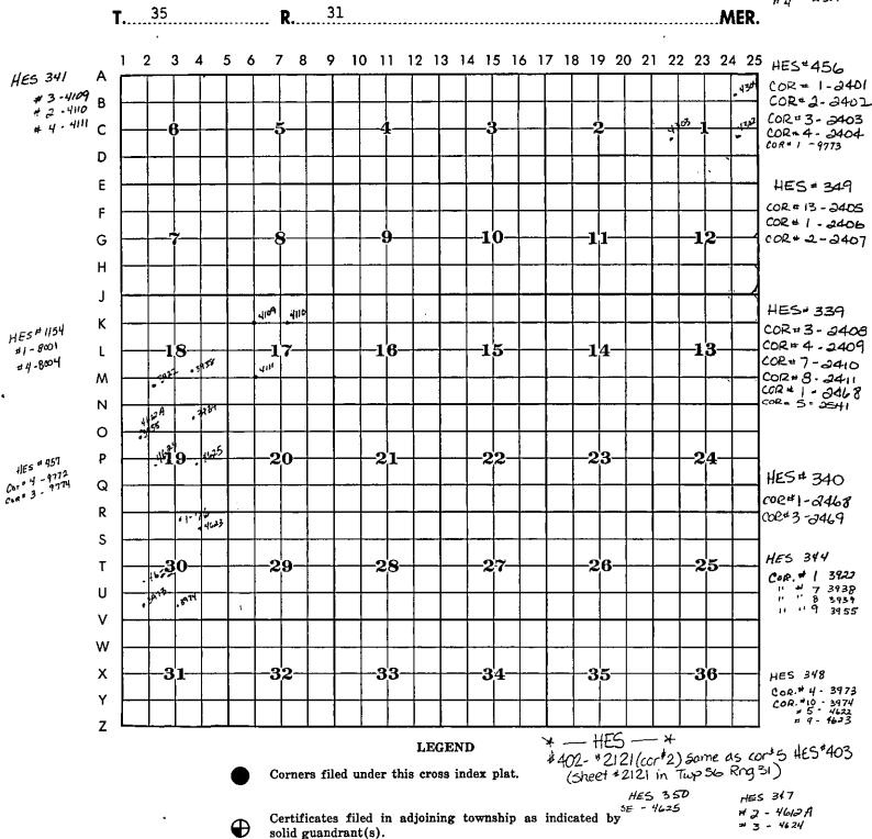
Each corner certificate is identified by an alphabetical-numerical coordinate number which is derived from the system shown on the township diagram. For example, the quarter-corner between Section 5 and 6 is identified as Corner C-5.
