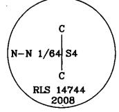
2. A 10" Douglas Fir bearing S 68° E at a distance of 27.1 feet and scribed (C-N-N 1/64 S4 BT).
