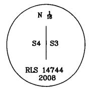
2. A 8" Douglas Fir bearing S 09° E at a distance of 32.1 feet and scribed (N 1/16 S3 BT).
