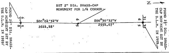
DIAGRAM OF CORNER: R26W T34N JAMES BURTON Surveyor's Seal N. 1-4 Cor certify that the information shown herein is true and correct Signature of Ground Party Chief STATE OF MONTANA M.L. HAIGES COUNTY OF LINCOLN certify that I have carefully performed or reviewed the work done on the diagrammed corner as reported on this recordation form and approve the same. Corner recorded on the sheet
