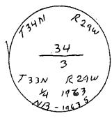
Set GI pipe, 1-1/8" diam., 28" long with brass cap marked as shown and established a new bearing tree 15" fir 60.4 feet N 44000' W of corner.
