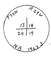
Set GI pipe, 1-1/8" diam. 28" long with brass cap marked as shown. Established following BT.
