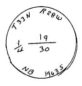
Set pipe with brass cap marked as shown:
