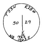
Set pipe with brass cap marked as shown.
