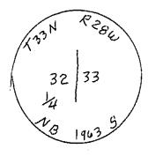
Set pipe with brass cap on side of stone marked as shown: Established new BT New BT 12" LPP mkd FSRM, bears N  $12^{\rm O}$  E 38 links
