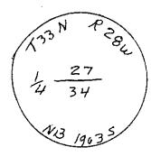
Set 2" x 36" pipe with brass cap in mound of stone with stone buried W side of pipe marked as shown. Established new BT.
