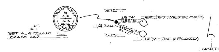
DIAGRAM OF CORNER: Surveyor's Seal I, KGRILEY
