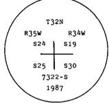
I buried the original stone on the east side of the new monument. Set a galvanized steel guard post with a Survey Marker decal attached, 3 ft. North of monument. I painted red bands around the bearing trees and attached BT and Land Survey Monument signs. I marked and scribed 3 new bearing trees:
