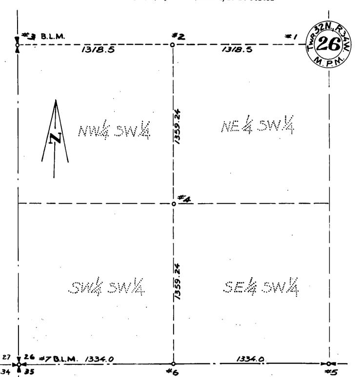
Cor. # 5 Replaced a post set by others with a Pipe from which a 24" Fir Bears S 45 W 62.4 Ft. Scribed S 262 Posted.A 14" Fir Bears N 65 W 20.3 Ft. Scribed 1. Posted
