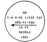
I set a reference monument, a 2 1/2 ins. dia. aluminum rod, 30 ins. long with attached 3 1/4 ins. dia. U.S.D.A. Forest Service aluminum cap, bears  $10^{\circ}28'08''E$ , 10 ft. dist., marked as shown
