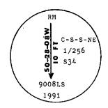
A cedar, 6 ins. dia., bears \$22°E, 39.6 ft. dist., mkd. X BT. A grand fir, 16 ins. dia., bears N81  $^{\circ}$ W, 23.0 ft. dist., mkd. C-S-S-NE 1/256 S34 BT.
