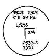
Set a  $2\frac{1}{2}$ " X 30" aluminum pipe with cap 24" in the ground. Raised a rock mound around cap from which a;
