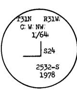
Set a  $2\frac{1}{2}$ " X 30" aluminum pipe with cap 24" in the ground. Raised a rock mound around cap from which a;
