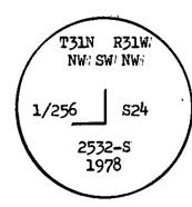
Set a  $2\frac{1}{2}$ " X 30" aluminum pipe with cap 24" in the ground. Raised a rock mound around cap, from which a;
