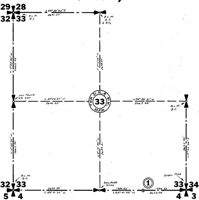
(1) Set a 5/8" by 24" Capped Steel Rod with no B.T.s cap Stamped: J.H.N. 4661 S.
