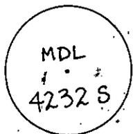
1-1/4 inch diameter yellow PVC plastic cap on 5/8 inch by 24 inch rebar.
