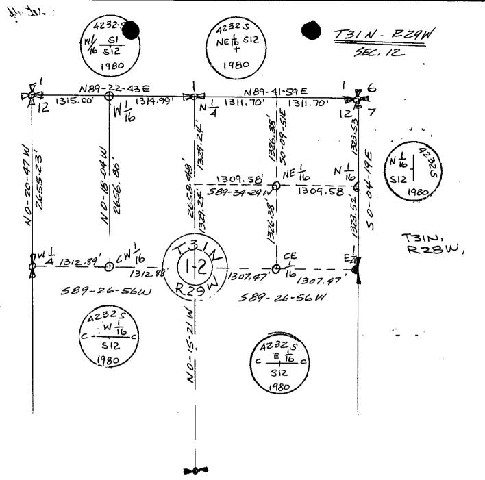
W 1/16 Set an aluminum pipe 2 1/2" X 30", 26" in ground, with cap marked as shown above for exact corner position From Which:
