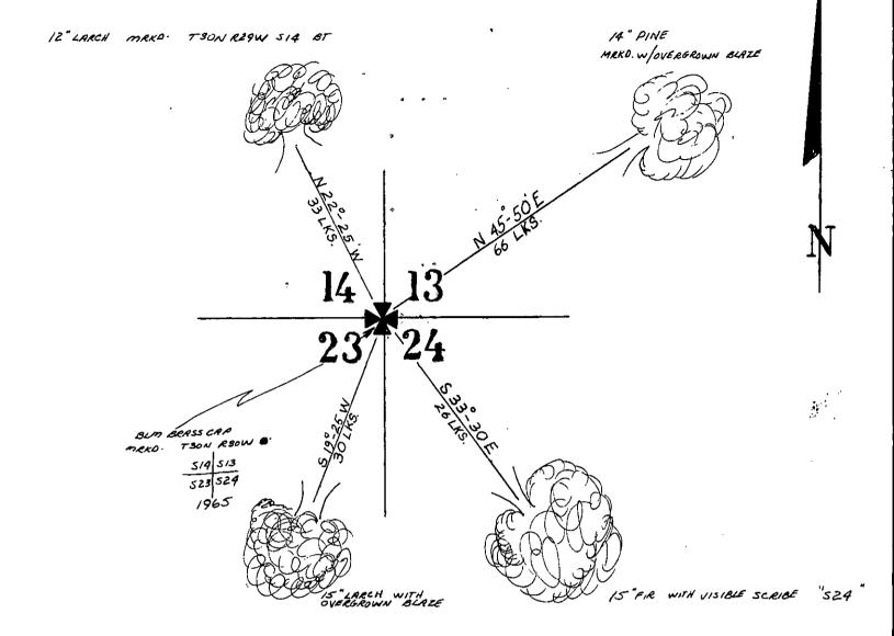
Record: 14" larch bearing  $S19\frac{1}{4}$ "W, 30 lks., with an overgrown blaze Found: Bearing tree alive and presently 15" in diameter
