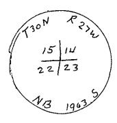
Set GI pipe  $1\frac{1}{2}$ " diam., 28" long with brass cap marked as shown and established new BT.
