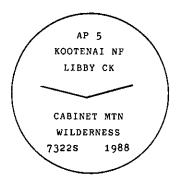
A larch, 11 ins. diam., bears  $868^{\circ}$ E, 8.0 ft. dist., marked with a snow blaze and a Locatioin Poster A 6 ft. galvanized steel guard post, south, 1 ft. dist., with a Wilderness Boundary decal attached.
