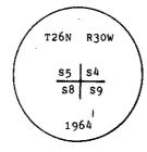
Bury the original stone alongside iron post. Established 4 new bearing trees as referenced below.
