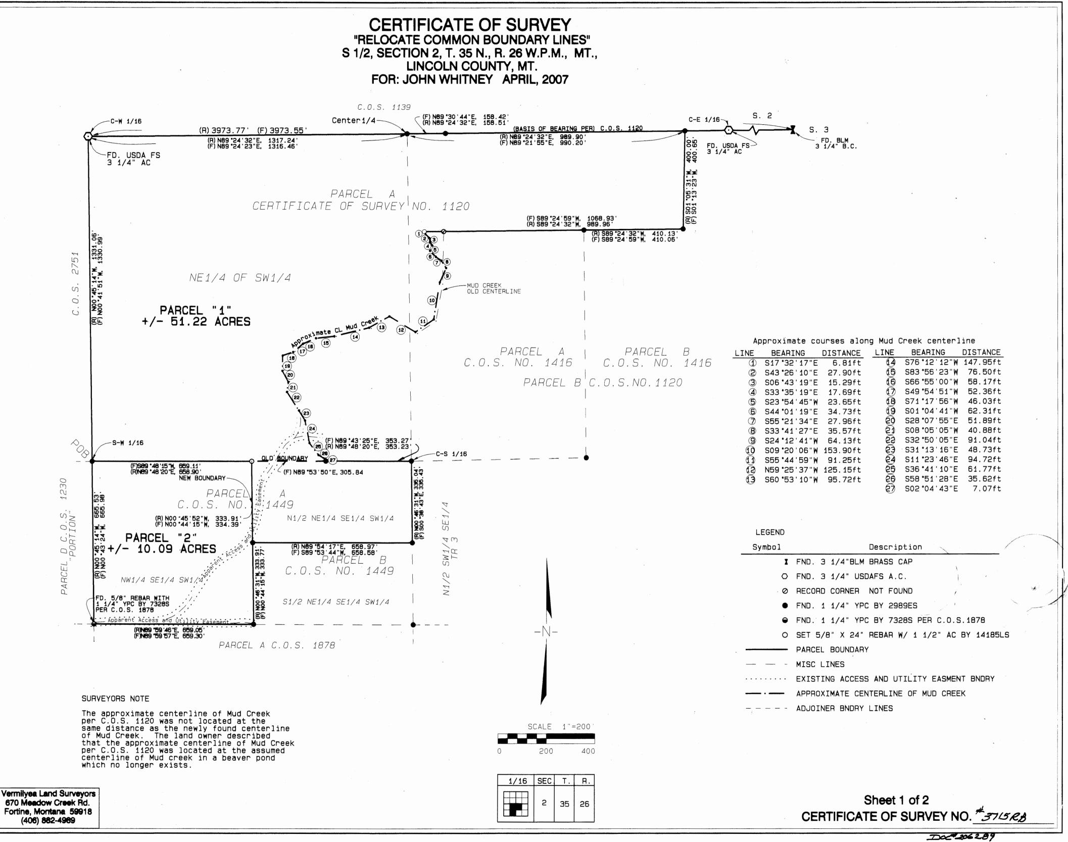
CERTIFICATE OF SURVEY "RELOCATE COMMON BOUNDARY LINES" S 1/2, SECTION 2, T. 35 N., R. 26 W.P.M., MT., LINCOLN COUNTY, MT. FOR: JOHN WHITNEY APRIL, 2007
