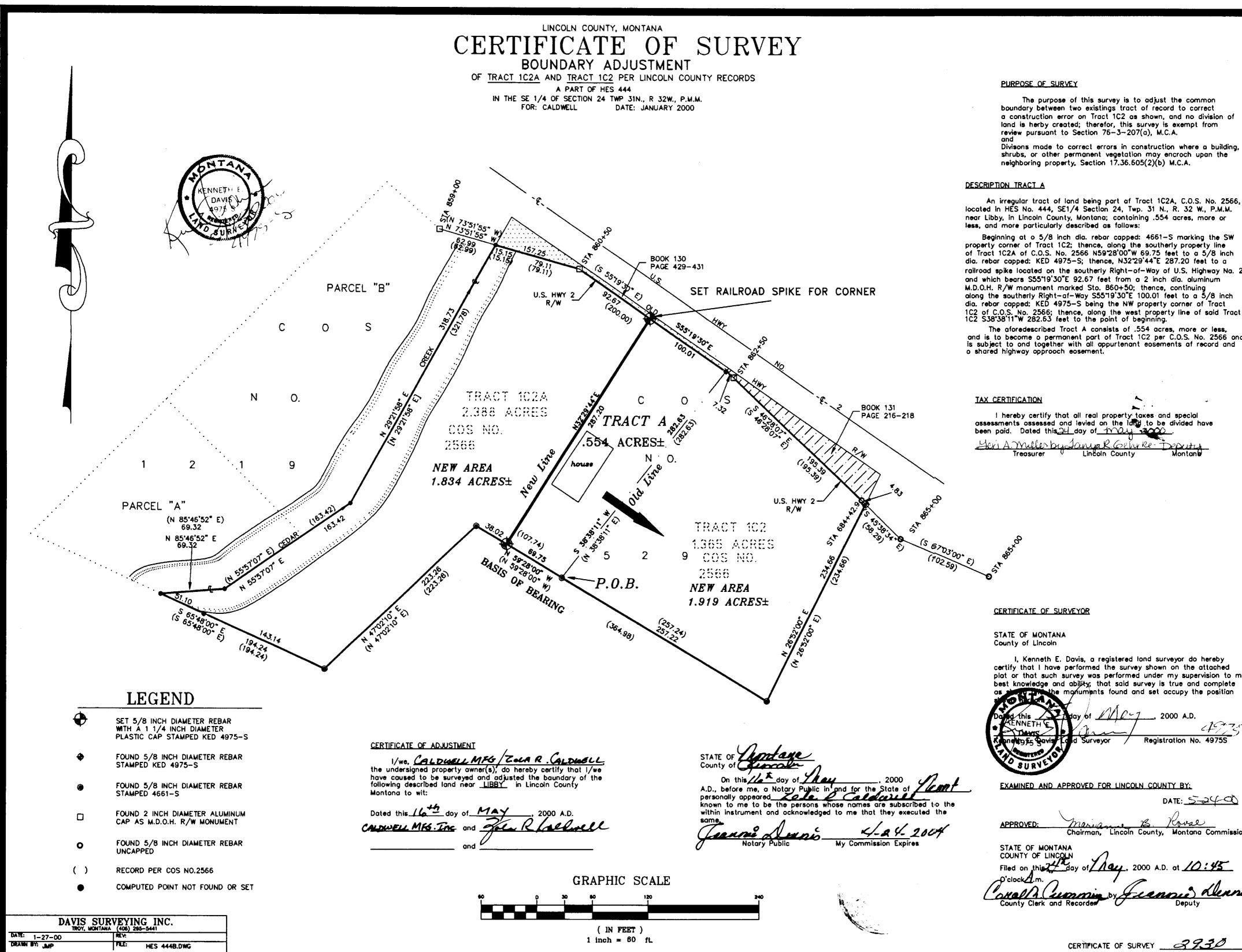
boundary between two existings tract of record to correct a construction error on Tract 1C2 as shown, and no division of land is herby created; therefor, this survey is exempt from review pursuant to Section 75-3-207(a), M.C.A.
