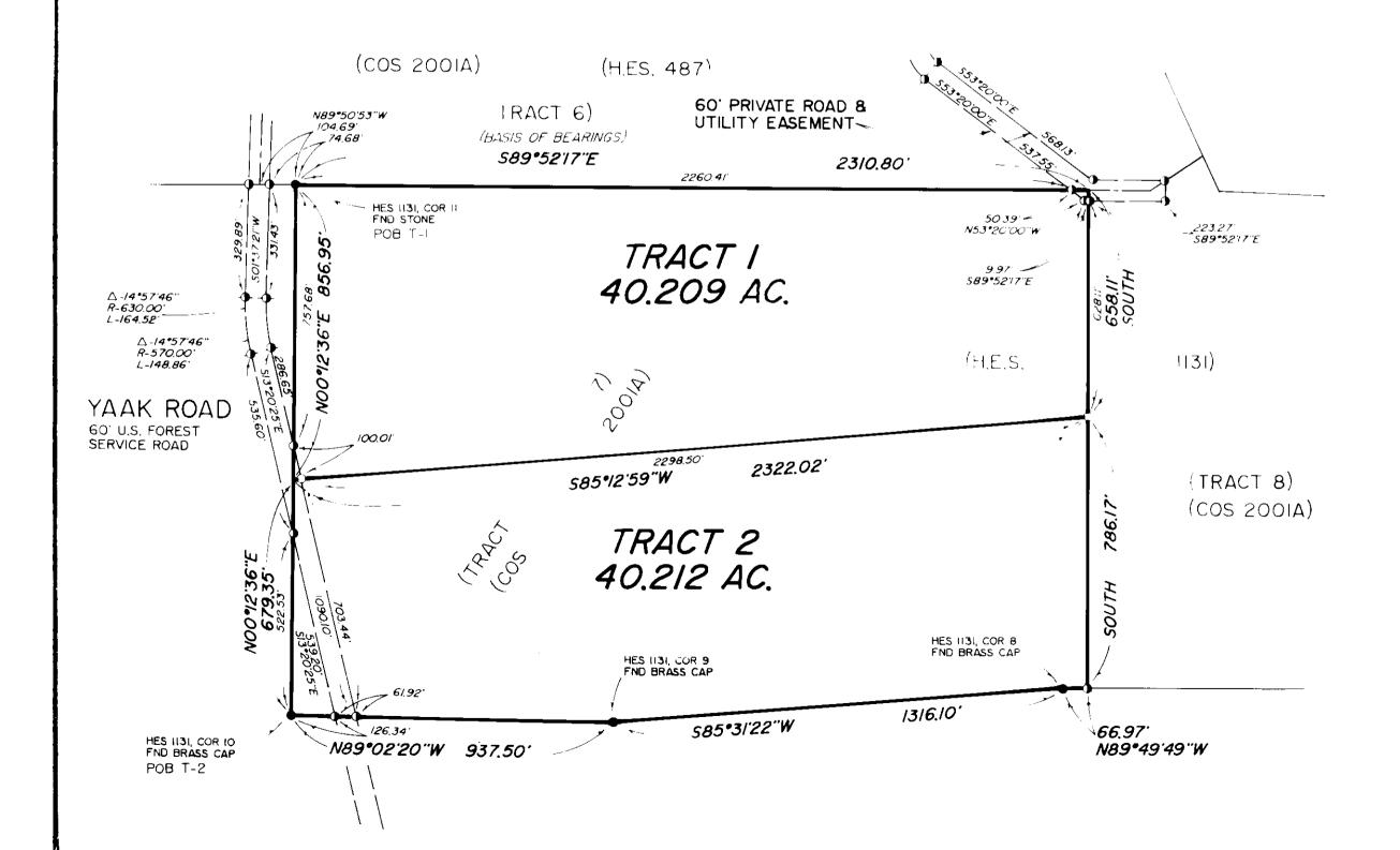
I SEC. COR. (AS NOTED) 2 1/4 CORNER (AS NOTED) 3 O CENTER SECTION (AS NOTED) 4. S I/16 CORNER (AS NOTED) 5. • FOUND (AS NOTED) 6 O SET 1/2" X 24" REBAR WITH I" PLASTIC CAP, STAMPED: SANDS, 7975-S 7. • FND 1/2" REBAR BY 7975-S CHAU CERTIFICATE OF SURVEYOR THOMAS E. SANDS REGISTRATION NO: 7975-5 STATE OF MONTANA ... COUNTY OF LINCOLN FILED ON THE STAY OF har, 1993 A.D. ATLINO O'CLOCK P. M CLERK & RECORDER SHEET OF SHEETS
