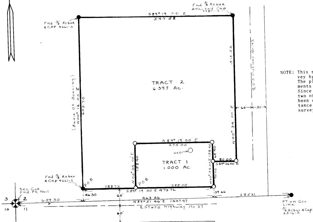
NOTE: This survey is taken from an unrecorded survey by Ninniman Engineering of Troy, Montana. The plat shows iron pins or concrete R/W Monuments on all corners adjacent to highways. Since the original survey, it is apparent that two of the R/W Monuments and 1 iron pin have been destroyed. I reset them at record distance and bearing as shown on the Ninniman survey.
