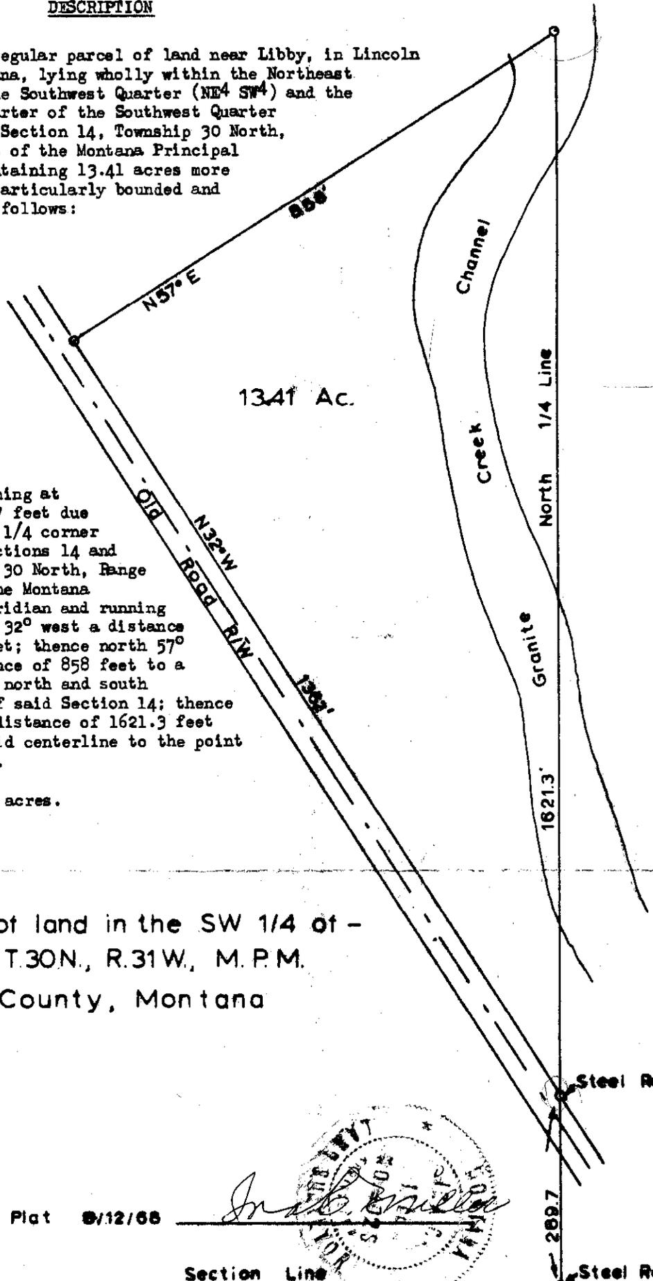
Beginning at a point 289.7 feet due north of the 1/4 corner common to Sections 14 and 23, Township 30 North, Range 31 West of the Montana Principal Meridian and running thence north 32° west a distance of 1362.0 feet; thence north 57° east a distance of 858 feet to a point on the north and south centerline of said Section 14; thence due south a distance of 1621.3 feet along the said centerline to the point of beginning.
