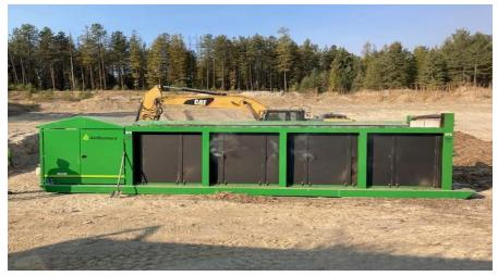
Lincoln County Solid Waste purchased an air curtain burner to help process wood waste while protecting our air quality. Landfill staff were trained in the safe and efficient operation and maintenance of the burner by a representative of the manufacturer in a two-day hands-on session at the Libby Landfill. This burner was purchased with grant funds.
