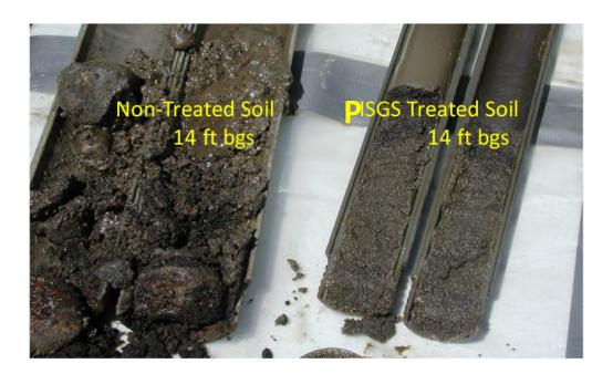
Photograph 1: Untreated Soil Core and ISGS treated soil core
